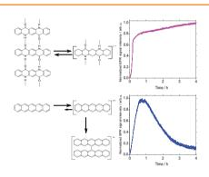
Air- and moisture-resistivity as well as chemical stability are key issues for organic electronics and thus, influence the operational lifetime of devices. The hydrogen-bonded pigment quinacridone is an example for extraordinary chemical stability. Here, spectroscopic studies on quinacridone as compared to pentacene thin-films confirm different spectral response of their radical cations, emphasizing the stability on quinacridone.
