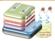
Water additive is incorporated into the perovskite precursor solution to control the oriented growth of crystal perovskites and improve the stability of perovskite solar cells. As a result, a power conversion efficiency of 16.06% and an improved cell stability under ambient conditions are achieved.
